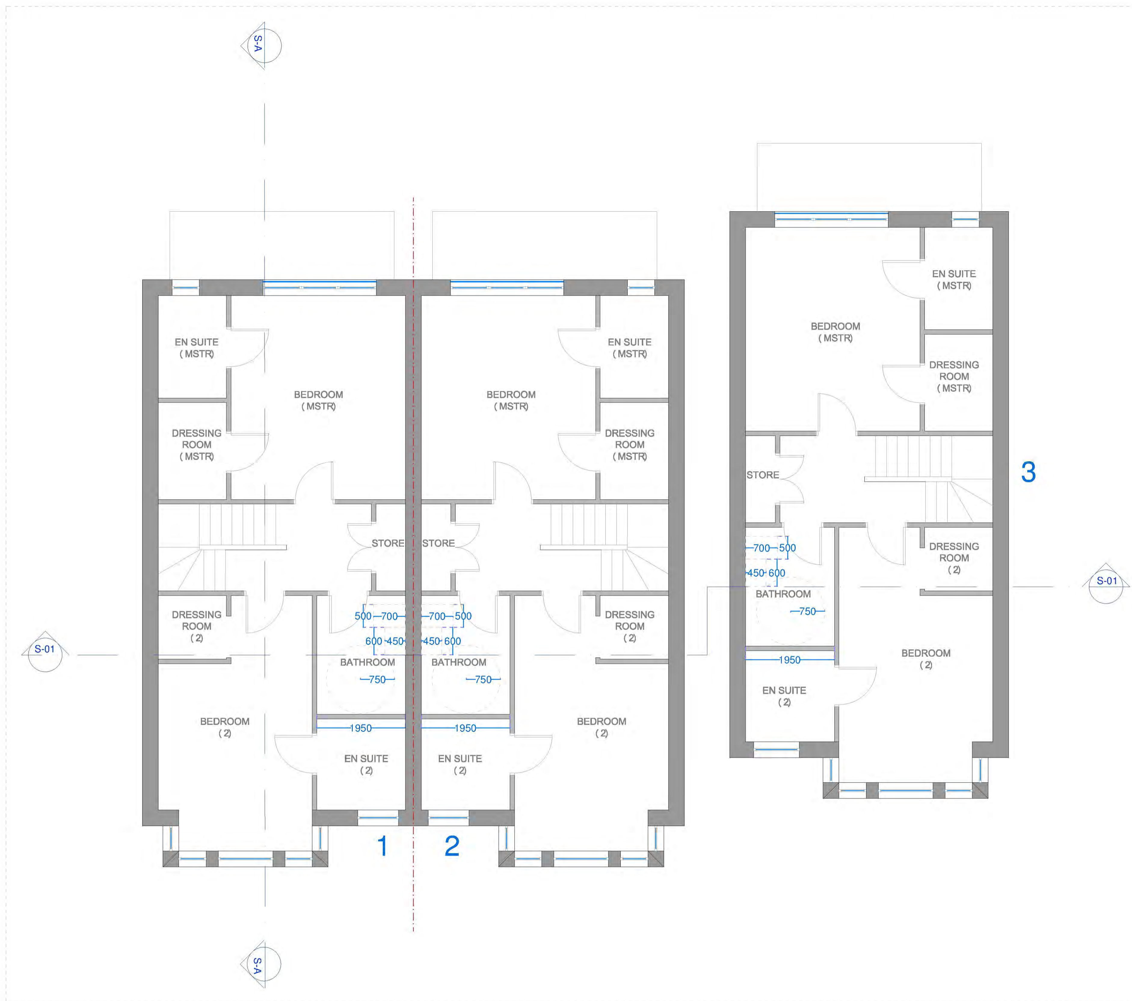
12 Proposed First Floor Plan GA Internal Floor Area 1 = 64sqm Internal Floor Area 2 = 64sqm Internal Floor Area 3 = 64sqm
